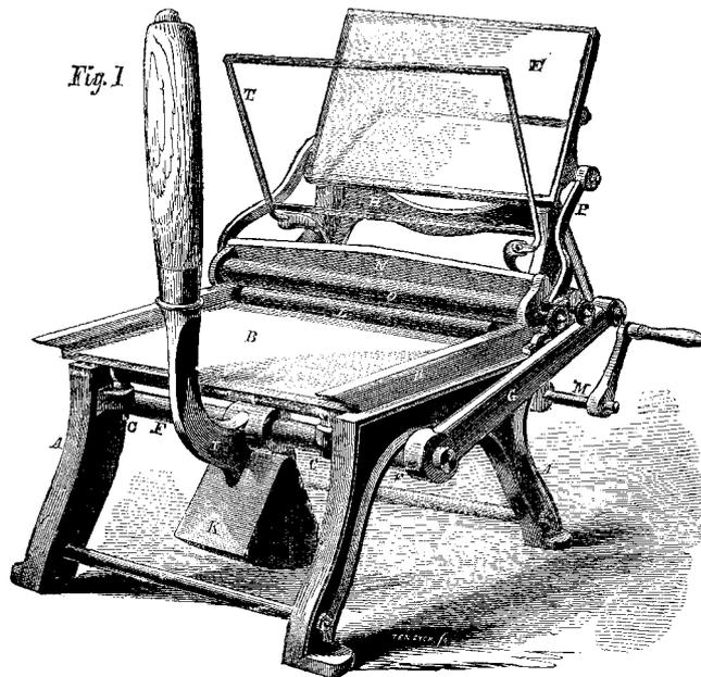
as to produce a very powerful impression on the form. On lifting I, all the motions are reversed, the levers G move backward, acting on H, to elevate the platen E, and while these parts are returning to their places, the rollers
