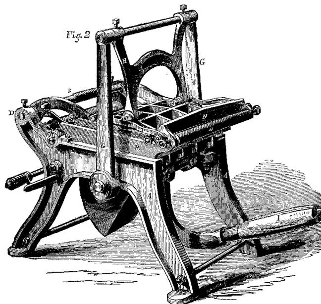
removed, and another to be substituted in its place. It will be observed that the inking rollers O, which are two in number, are compelled by the motion of N to travel twice across the form—once, as the platen is brought down, and again as the platen is elevated—so that the types are liberally and uniformly inked as by the ordinary arrangement, and the whole operation is conducted not only rapidly and easily, but with a very high degree of
