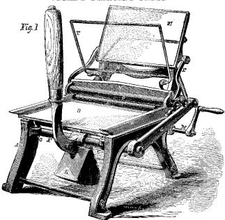
as to produce a very powerful impression on  $\begin{bmatrix} 0 \\ o & a \\ for a new impression \\ As the platen E recedes \\ for a new impression. As the platen E recedes \\ \end{bmatrix}$ reversed, the levers G more backward, acting into the position represented in Fig. 1, it on H, to elevate the platen E, and while these leaves the frisket T in the position indicated, parts are returning to their places, the rollers and allows the printed sheet to be readily
