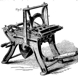
place. It will be observed that the inking rollers O, which are two in number, are compelled by the motion of N to travel twice across the form-once, as the platen is brought down, and again as the platen is elevated-so that the types are liberally and uniformly inked as by the ordinary arrangement, and the whole operation is conducted not only rapidly press in operation, working very rapidly, and easily, but with a very high degree of There are many points in this machine, among
